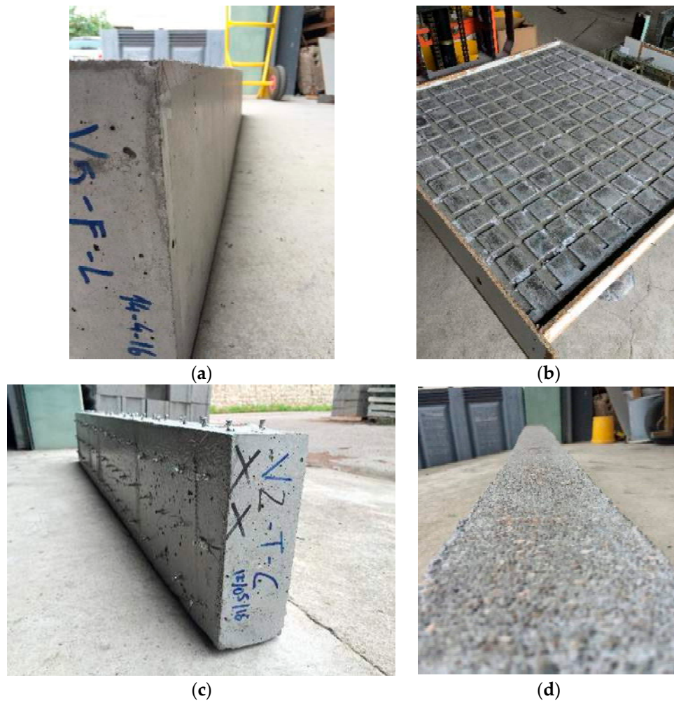
Figure 9. Different surface conditions for the interface between the cover and the bulk of RC members: (a) Smooth; (b) Indented; (c) Smooth with micro connectors; (d) treated with water jet.
