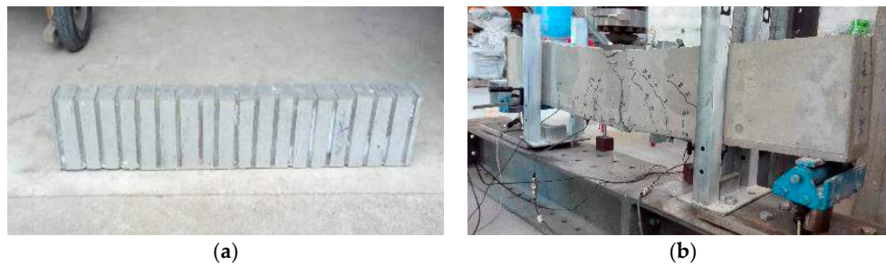
Figure 10. (a) Beam with indented surface; (b) Beam's test.
